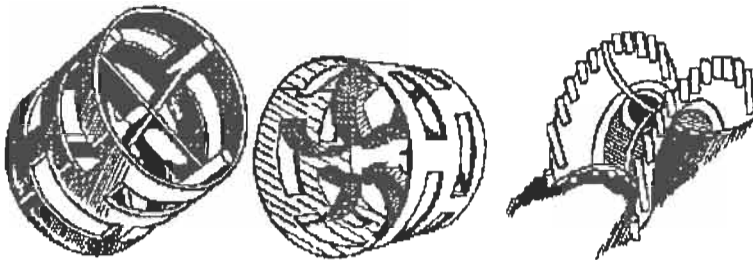
Figure 6. Sketch of common packing configurations.
